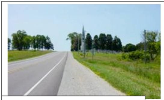
(Q8) Shoulder – paved section + unpaved section
