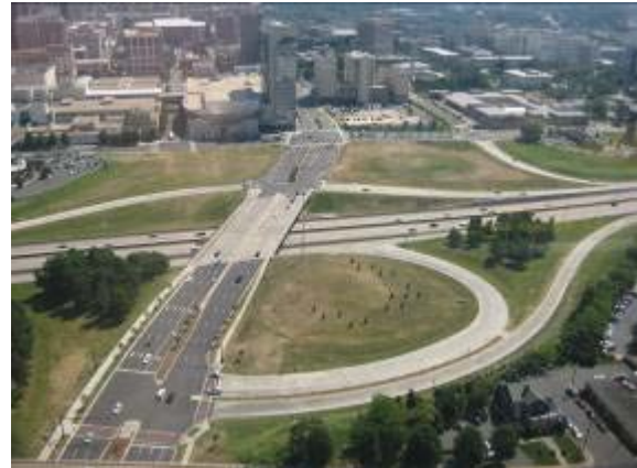
The aerial photo above shows how Charlotte’s rebuilt I-277 interchange helped reconnect surrounding surface streets; improved walkability with sidewalks, crosswalks and medians; and created redevelopment sites connected to downtown (the grassy areas at top of photo have been offered for sale to developers).
